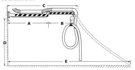
Note: Recommended mounting elevation above the finish floor (AFF) should be determined for each application. Total hose reach will vary based on mounting elevation and length of end hose. Designer must confirm that the BRL or BRC-450 recoil balancer can lift and recoil the hose weight and length required.
